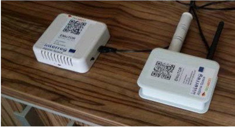
Figure 3: ENIoT sensor box-Arduino (left) and data concentrator-Raspberry Pi (right) [Source: THE4BEES archive]
